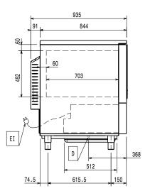
Drain Electrical inlet (power)
